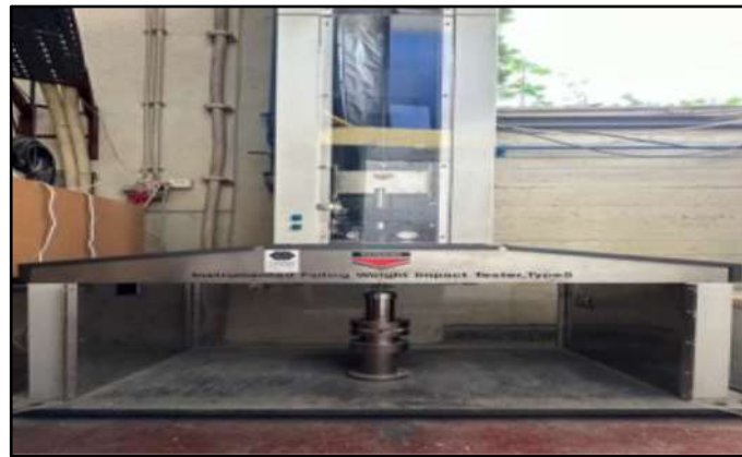
Figure 4: Low velocity Impact testing machine
