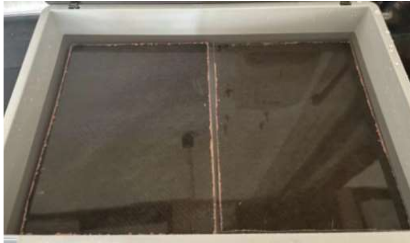
Figure 2: Treated specimen for water absorption
