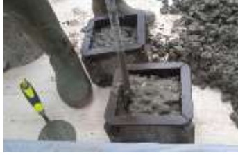
Fig 4: Compacting the concrete in the cube mould
