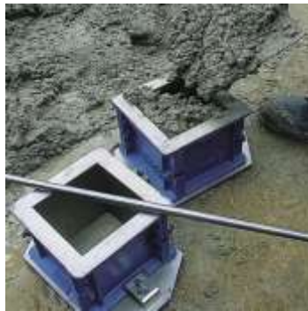
Fig 3: Filling the mould (for 150 mm cube 3 equal layers)
