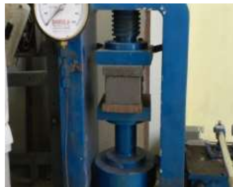
Figure 9: Testing of 10%MSW specimen at 7 days curing
